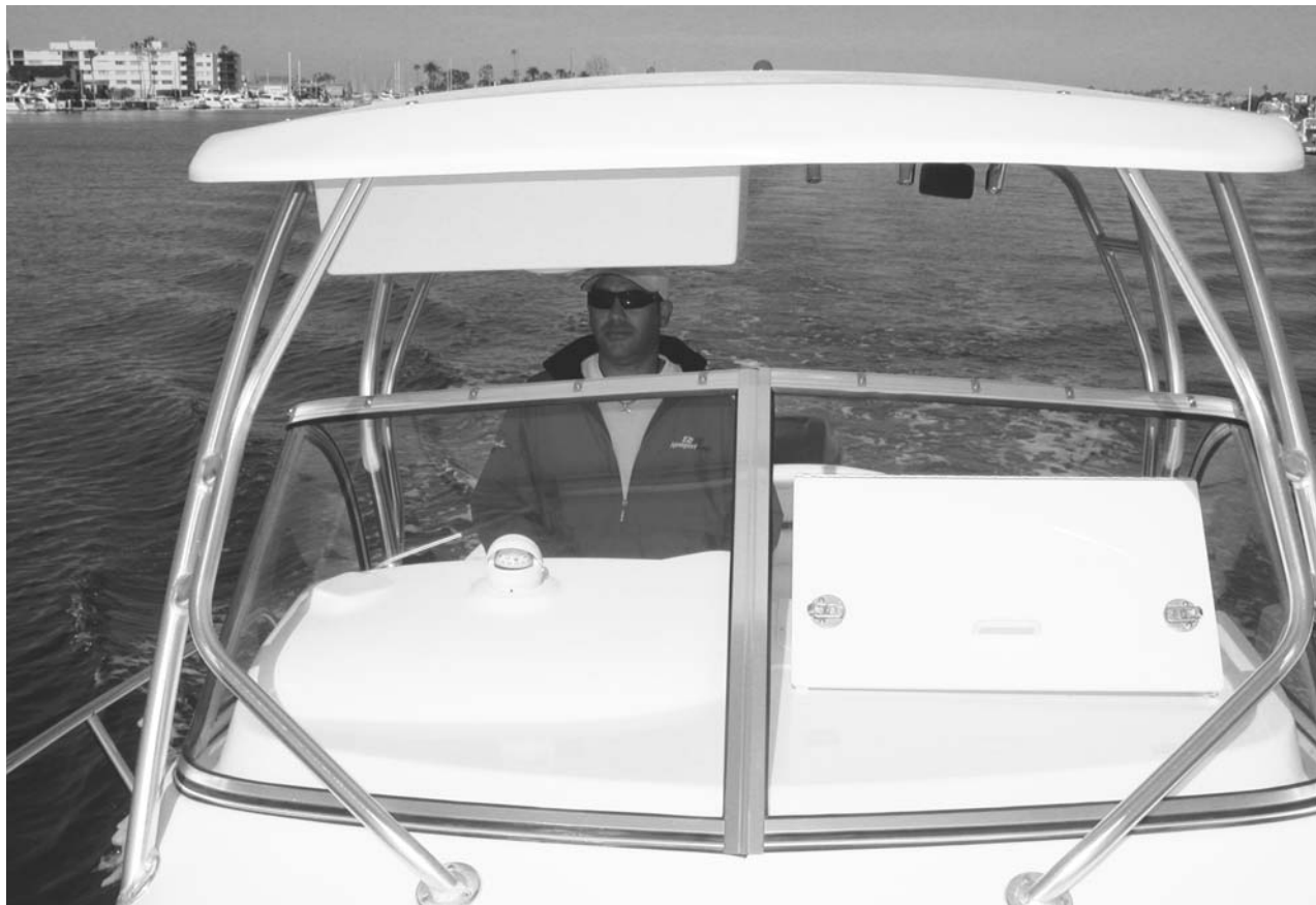
THE WRAP-AROUND WINDSHIELD protects passengers from the elements, and snaps allow for the conversion to a fully-enclosed Isinglass cockpit.
